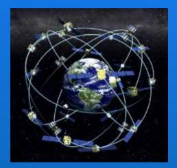
GPS system consists of around 27 active satellites of which 24 are normally in operation. Normally reception of 3-4 gives good location.
