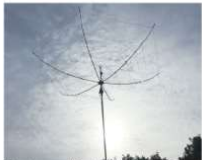
The hex beam was assembled and mounted on a rotator and portable mast.
