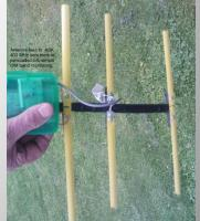
Build it: 2 meter Tape Measure Yagi Beam Antenna
